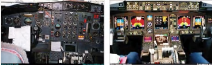
Initial design of the airplane cockpit (left); the digital design of the airplane cockpit (right), which has taken human factors into account.
